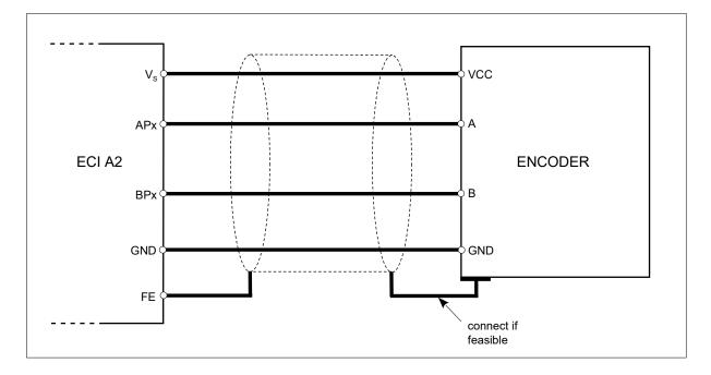
Due to high levels of noise usually found in harsh industrial environments, the use of shielded cable is highly recommended; the sheath should be tied to the FE pin available on the connector. Leaving the shield unconnected greatly impairs the shielding performances of the cable, leading to a worsening of the signal to noise ratio.
