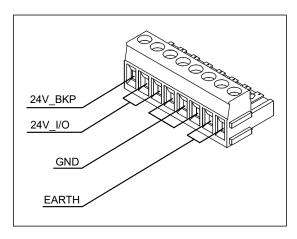
of detrimental ground loops, the ground contact should be earthed only once in the electrical cabinet, and the impedance of the earth connections should be kept low enough to effectively drain RF noise.
