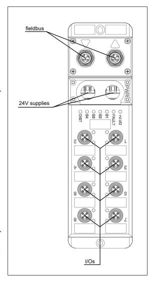
(e.g. an emergency button or a door switch). If the user doesn't need this feature, the two supplies can be shorted together.
