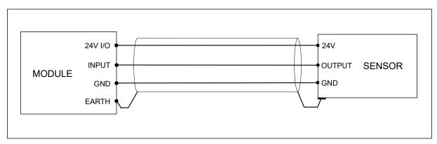
In this example, a shielded cable is used for the wiring. Even if not absolutely necessary in many applications, the use of shielded cable is very effective in reducing electrical noise picking up, especially in harsh industrial environments. The sheath should be grounded at the module side, and also at the sensor side whenever possible.
