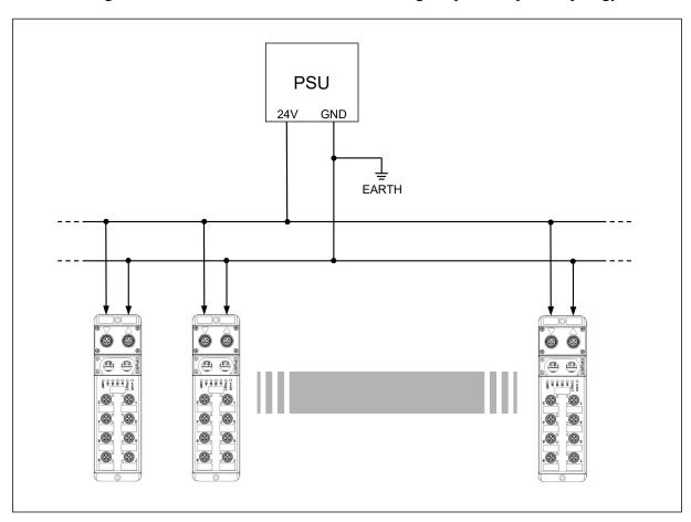
An example of daisy-chain topology is instead depicted in the following illustration; for simplicity, in each example only one PSU is shown. Whenever necessity of split power
