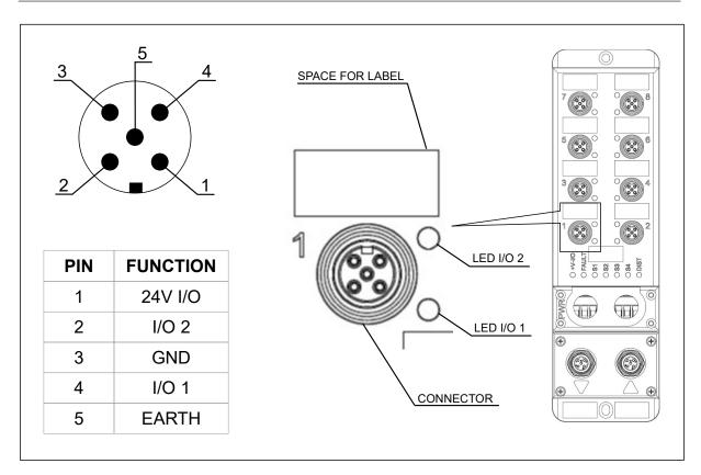
Each connector, of the widely-known industry standard M12 type, carries two I/Os, their ground and a 24V I/O power supply (used to eventually feed sensors). In case of an overload or a short circuit, an internal 5 x 20 mm fuse protects the cables and the electronics. The center pin is tied to earth, and is used to connect the outer sheath of shielded cables.
