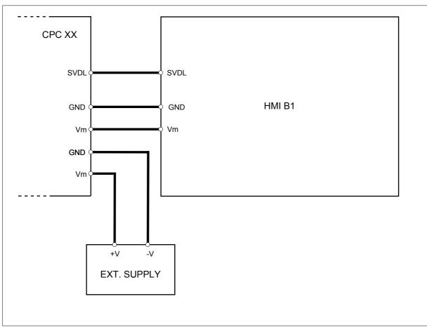
SDVL and power supply cables connecting CPC XX and HMI B1 must have the same length and should be bundled together.
