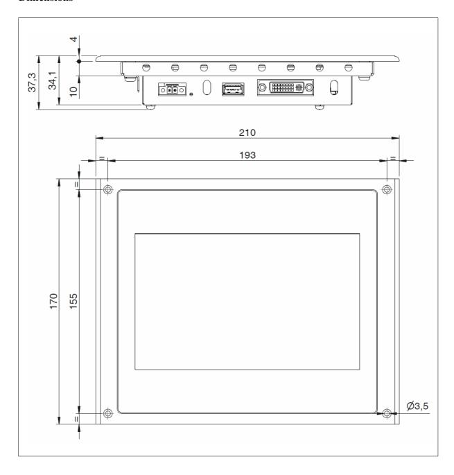
The module HMI B1 needs to be fixed on a stable and rigid panel provided with 4xM3 metal threaded hole, min. 1.5mm deep. Use 4xM3x10mm Fe/Zn (not countersunk head type) screws, min. class 8.8, tightened at 1Nm.
