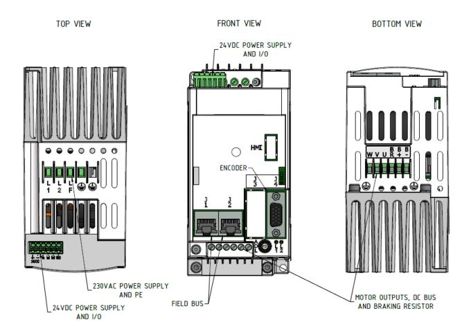
The release code KZ010375 is also equipped with a stage for piloting the brake resistor.
