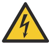
The servomotor generates high earth leakage current; do not power the servomotor without PE (Ground) connection, to avoid the risk of Electric Shock if you touch metal components (such as the heat sink).
