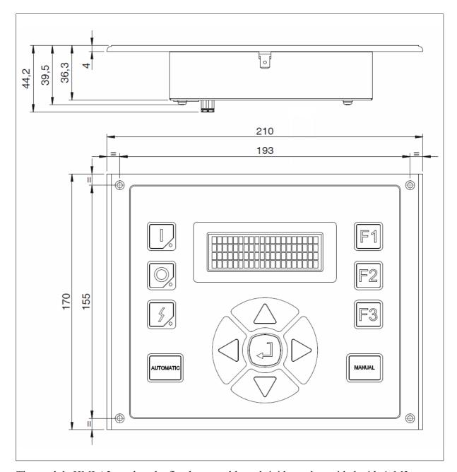
The module HMI A2 needs to be fixed on a stable and rigid panel provided with 4xM3 metal threaded hole, min. 1.5mm deep. Use 4xM3x10mm Fe/Zn (not countersunk head type) screws, min. class 8.8, tightened at 1Nm.
