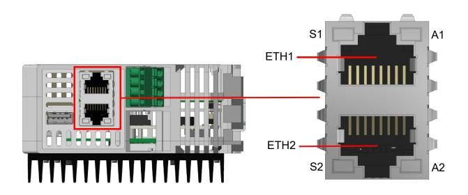
Each Ethernet port has two LEDs. The first, marked by the letter S, indicates the communication speed of the port involved. It is a two-color LED (green / orange); according to the speed at which the Ethernet port is communicating, the LED takes on a different color. The second, marked by the letter A, indicates the state of activity of the port itself, or if the port is connected or if it is communicating.
