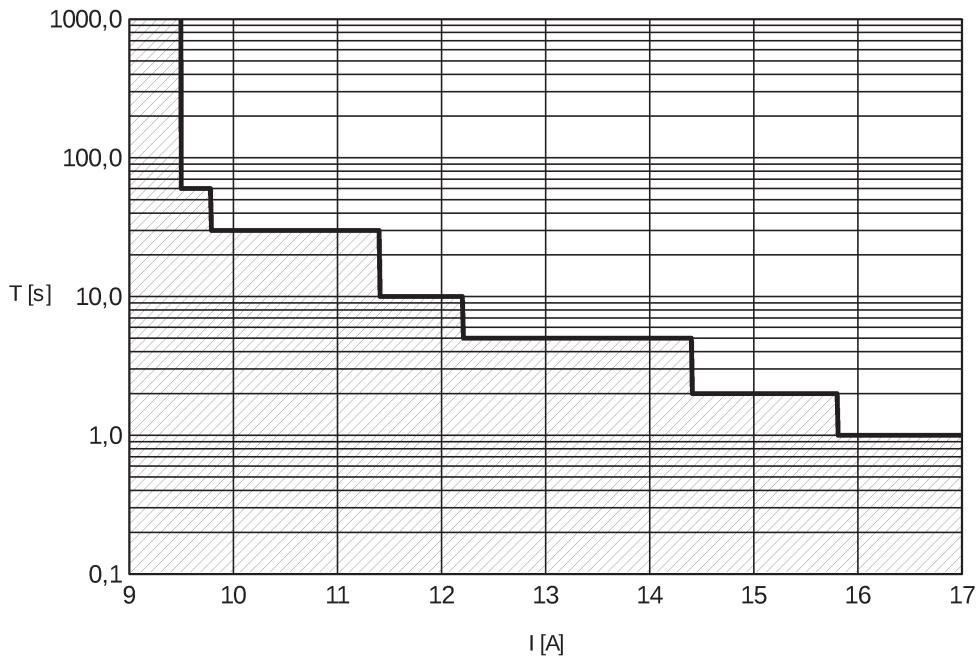
The curves refer to gPV 10x38 fuse-links. More precisely, the overload diagnostic intervenes earlier than the fuse, provided the rated current of the fuses in use is equal to 12A (single-phase) and 20A (three-phase). The fuse blows only in case of short-circuit or heavy overload, thus avoiding its interruption during normal operation.
