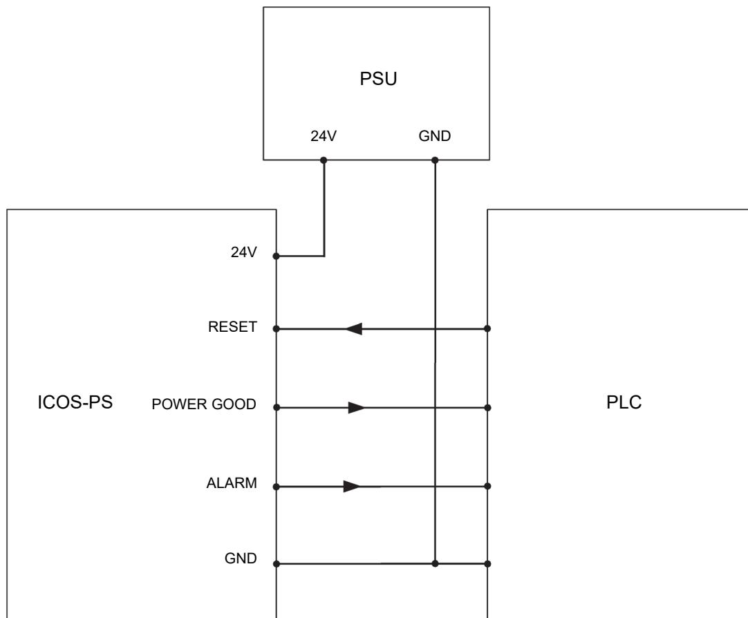
These inputs and outputs are suited for 24V digital signals, in order to be able to interface with standard industrial electronics (in particular PLCs).
