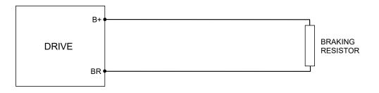
The bus voltage is available on the terminal board (contacts B+ and B-), for connecting a servodrive/inverter battery in parallel. This connection is advantageous form the standpoint of power dissipation in the braking resistors, because a portion of the power generated during braking can be used by another servodrive/inverter, instead of being dissipated in the braking resistor.
