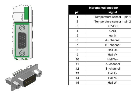
The interface for the Hall sensors is only provided on version that can also pilot brushless motors. Carefully check the signal polarity before connecting the encoder; otherwise, the motor might rotate uncontrollably. Risk of electrical and/or mechanical damage to the system.
