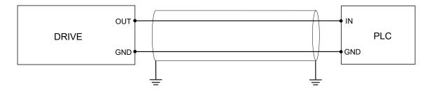
In this case, electrical interference problems are more likely, therefore it is recommended to use a shielded cable for the connections. The shield must be connected to earth on both sides, preferably with low-impedance connection, such as a metal cam; the shield is totally ineffective if it is left floating.
