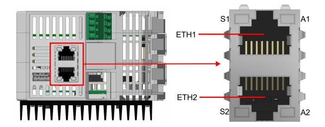
Each Ethernet port features two LEDs: the first one, identified by the letter S, indicates the communication speed of the concerned port. It is a bicolor lamp (green/orange); it changes its colour according to the communication speed of the Ethernet port.
