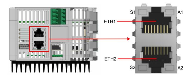
Each Ethernet port features two LEDs: the first one, identified by the letter S, indicates the communication speed of the concerned port. It is a bicolor lamp (green/orange); it changes its colour according to the communication speed of the Ethernet port.
