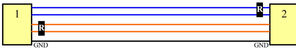
Example of RS422 wiring
