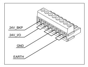
equipotential with earth; to avoid the generation of detrimental ground loops, the ground contact should be earthed only once in the electrical cabinet, and the impedance of the earth connections should be kept low enough to effectively drain RF noise.
